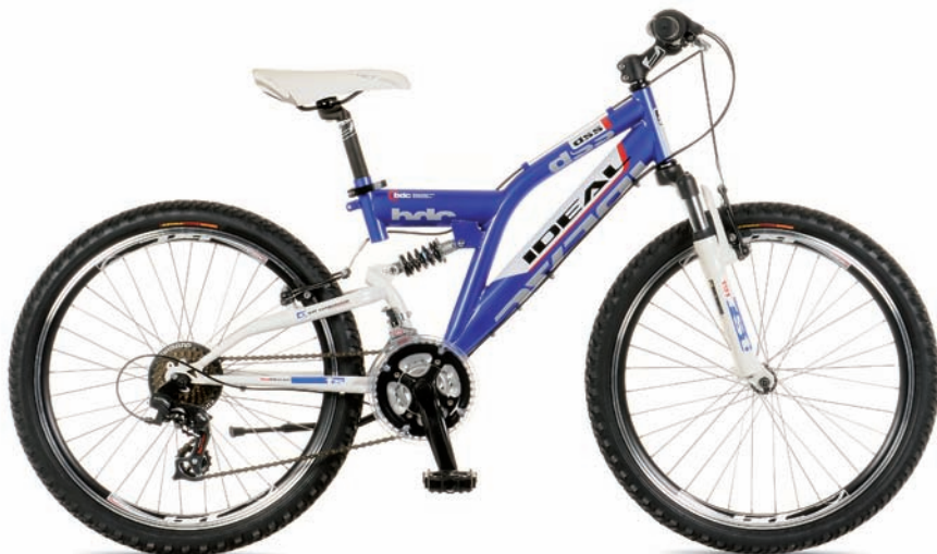
DSS WHEEL 24" SPEED 21 FRAME HI-TEN, 37cm FORK / SHOCK RST 191, ALLOY CROWN, 50mm / COIL SHOCK, 500lb/in TRANSMISSION SHIMANO RD-TX31, SL-RS35 & 7sp. MF-TZ 14/28T BRAKES COLD FORGED V-BRAKES WHEELS ALLOY QR HUBS, KENDA 1.95 TIRES
