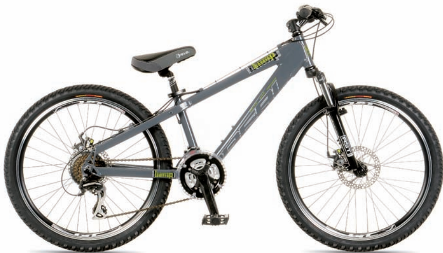
AXION WHEEL 24" SPEED 21 FRAME ALLOY-6061, ACTIVE GEOMETRY, 38cm FORK RST 191, ALLOY CROWN, 50mm, COIL SHOCK, 500lb/in TRANSMISSION SHIMANO ACERA RD-M360, ST-EF50 & 7sp. MF-TZ 14/28T BRAKES MECHANICAL DISCS or COLD FORGED V-BRAKES WHEELS ALLOY QR HUBS, KENDA 1.95 TIRES
