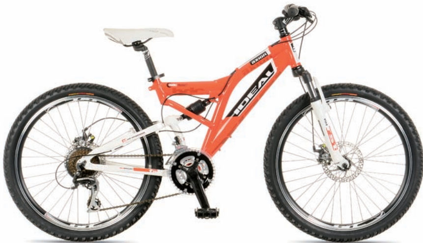
AXION WHEEL 24" SPEED 21 FRAME ALLOY-6061, ACTIVE GEOMETRY, 38cm FORK RST 191, ALLOY CROWN, 50mm, COIL SHOCK, 500lb/in TRANSMISSION SHIMANO ACERA RD-M360, ST-EF50 & 7sp. MF-TZ 14/28T BRAKES MECHANICAL DISCS or COLD FORGED V-BRAKES WHEELS ALLOY QR HUBS, KENDA 1.95 TIRES
